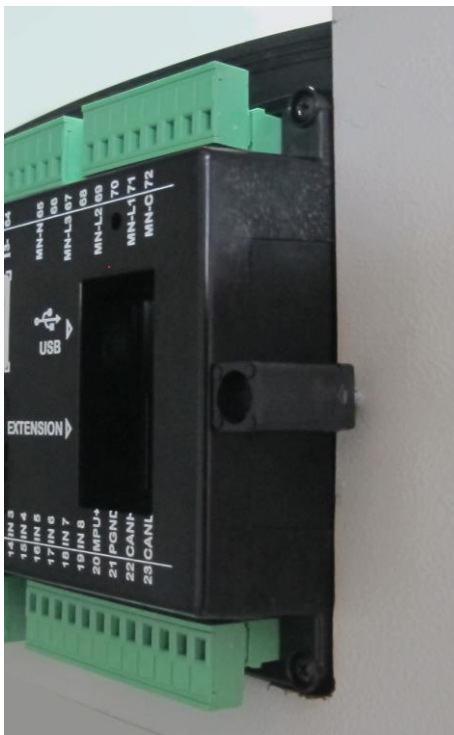
Installation of screw type bracket
